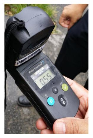
Free chlorine at terminal water 30km away from WTP: 0.55ppm
